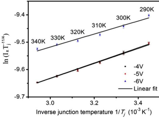
Fig. 2. The  $T_j$  dependence of  $I_R$  under different  $V_R$  values for B3 LED.
